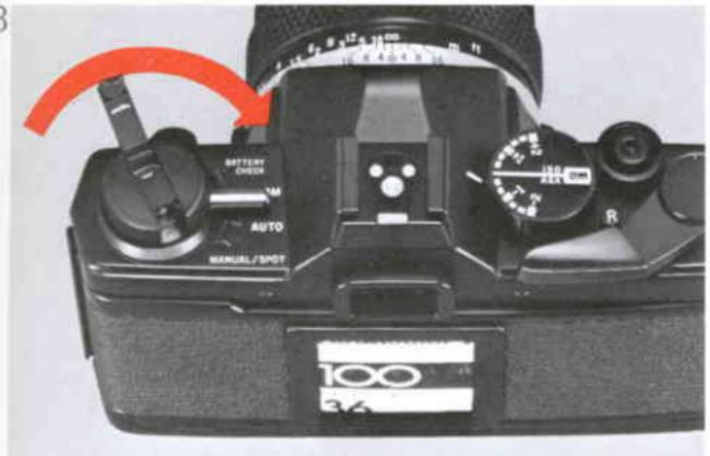
**E** Fold out the rewind crank and wind it until the film tension is released.
