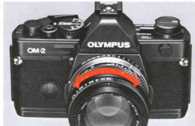
**E** Press the shutter release slightly to turn on the viewfinder. (A built-in battery conserves power by turning off the viewfinder display after 120 seconds.)
