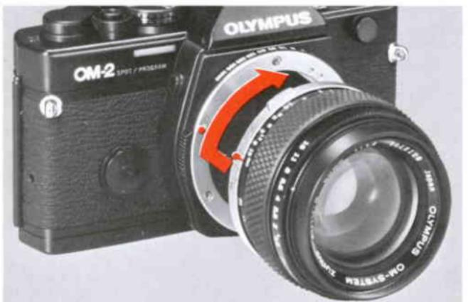
**E** Align the red dots and rotate the lens clockwise until it locks.
