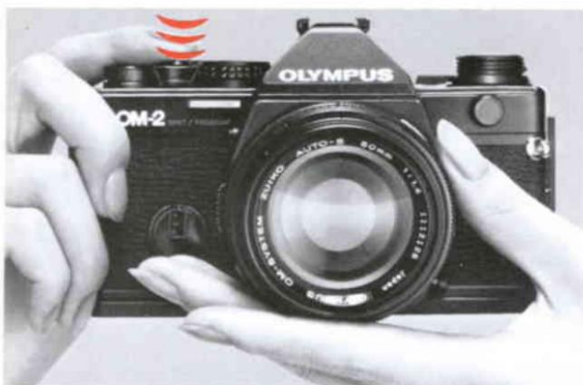
**E** Press the shutter release slightly to turn on the viewfinder. (A built-in battery conserves turns off the viewfinder display after 120 sec.)
