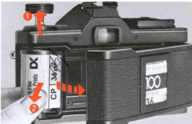
**E** Open the camera back by pulling up on the rewind knob and remove the film.
