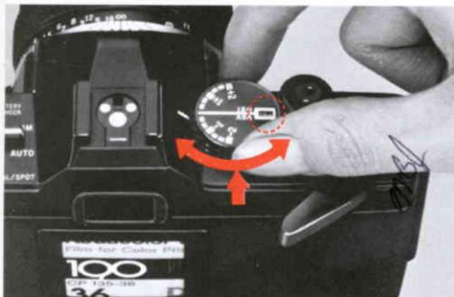
**E** Lift up the outer collar and rotate until the ISO speed appears in the window.
