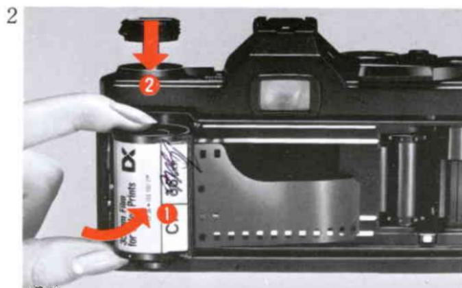
**E** Place the film cartridge in the film chamber.
